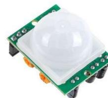
Fig.3 Motion sensor
